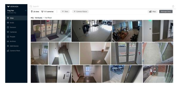
Command, Verkada's cloud-based management software, is designed to deliver simple access and management for all cameras and users across all sites from virtually anywhere in the world. From Command, users can set up new cameras, create new sites, manage settings, access live and archived footage, manage users, and access the advanced features powered by Verkada's edge-based analytics.
